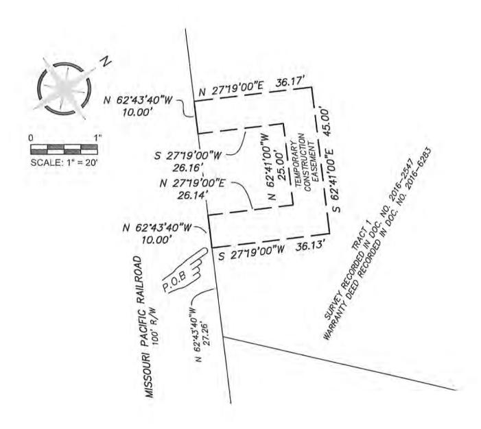
BEARINGS ARE REFERENCED TO MISSOURI STATE PLANE COORDINATE SYSTEM (NAD 1983) CENTRAL ZONE.
