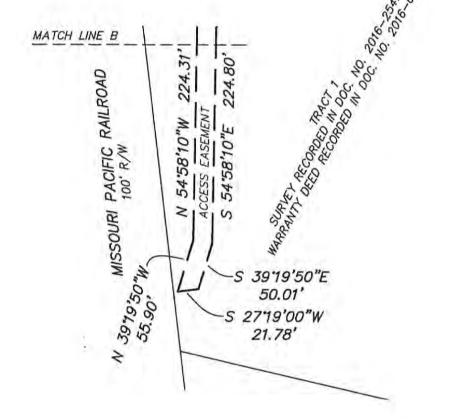
BEARINGS ARE REFERENCED TO MISSOURI STATE PLANE COORDINATE SYSTEM (NAD 1983) CENTRAL ZONE.
