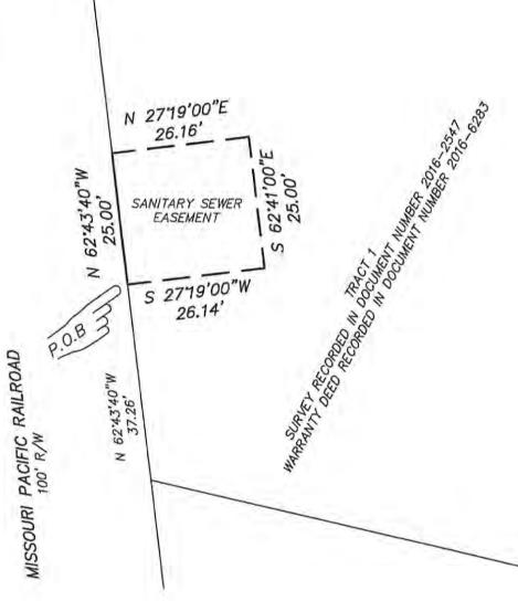
BEARINGS ARE REFERENCED TO MISSOURI STATE PLANE COORDINATE SYSTEM (NAD 1983) CENTRAL ZONE.
