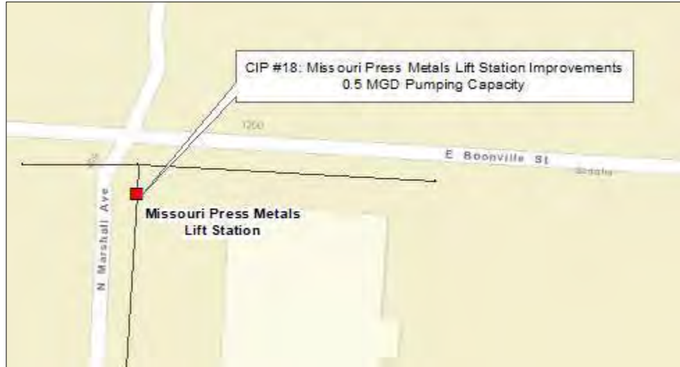
Figure 8-17: CIP #18 - Missouri Press Metals Lift Station Improvements
