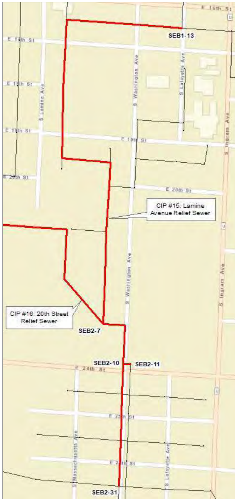
Figure 8-14: CIP #15 - Lamine Avenue Relief Sewer
