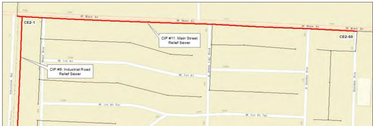
Figure 8-10: CIP #11 - Main Street Relief Sewer
