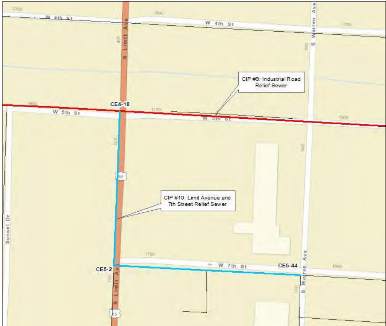
Figure 8-9: CIP #10 - Limit Avenue and 7 th Street Relief Sewer
