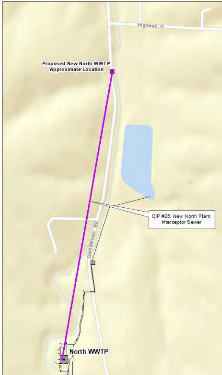
Figure 8-20: CIP #25 - New North Plant Interceptor Sewer
